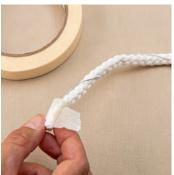
**4.** Wrap a length of masking tape around the ends to keep the steel wire in place
