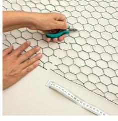
**2.** Cut a square piece of chicken wire. Use wire-cutters. Cut into the same mesh row.
