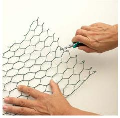
**3.** Make hooks on one side of the chicken wireusing flat-nosed pliers.
