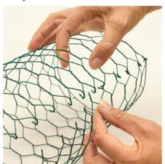
**4.** Roll the chicken wire to form a tube. Use your fingers and flat-nosed pliers.
