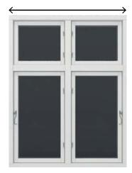
**1.** Measure how wide your window is. Add about 20% or 20-30 cm more to the window width. Cut the rail to fit your desired dimensions.
