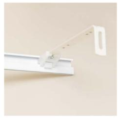
**4.** Push the bracket into the rail from the end, the brackets should be spaced max 50 cm apart
